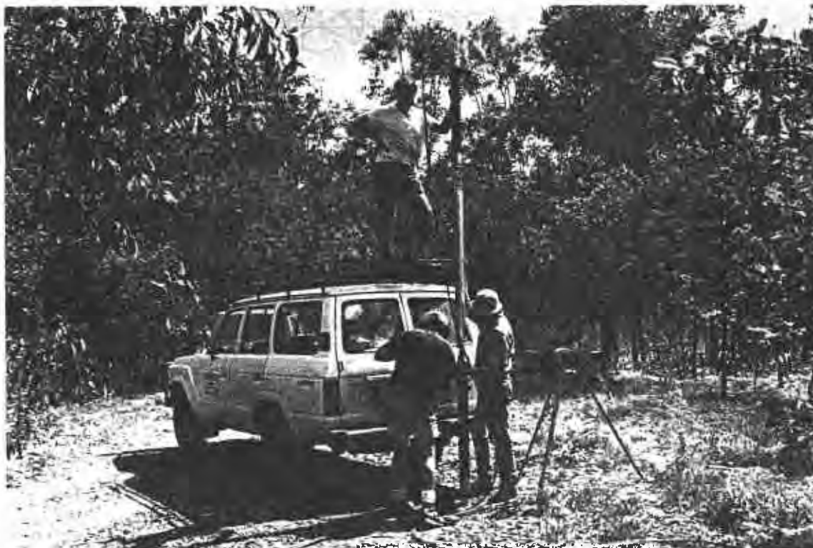
Figure 3.20 Various methods of obtaining water samples were used. Here a double packer (black sections at each end) pump system is being prepared for lowering down PH 15 on grid-line 6048 mN. Work was mostly done during the "dry" season—the dry brown "spear" grass attests to the intense seasonal aridity and high temperatures (around 35°C).
